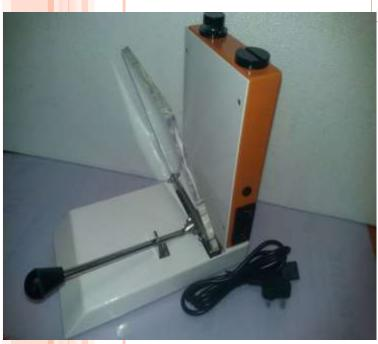
Plasma Extractor is designeed to **Extract Blood component from** centrefuge Bags. The spring loaded front panel applies pressure on the collected bag cousing the liquid to contain in transfer bag. Its sturdy construction makes it durable, easy to use and portable, the unit is available in both version automic and manual.
